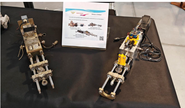
Virtu'Ailes display The display showed items removed from the simulator, like this sample hydraulic jack for the flight controls, and a spare of the electronic jacks that were previously fitted. Photo: Virtu'Ailes
