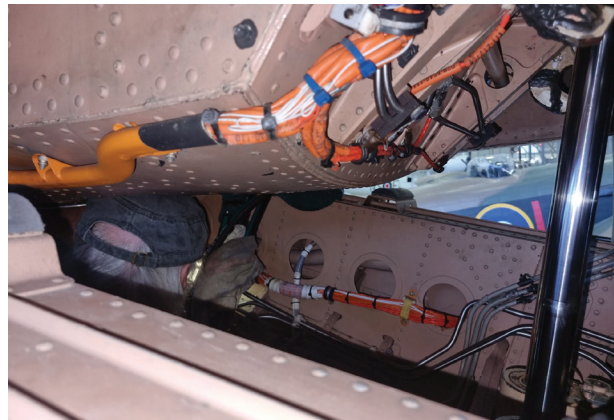
Working on the mechanism Peter Ugle at work on the interior of the nose hinge. Photo: Heritage Concorde
