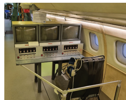
Observer's station The central console of the observer's station in the cabin; the perspex cover has been removed so that work can be done on the bulbs and captions. Photo: Heritage Concorde
