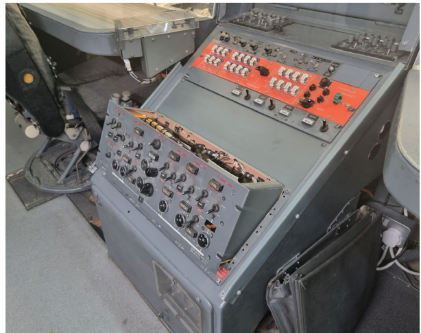
Observer's station The central console of the observer's station in the cabin; the perspex cover has been removed so that work can be done on the bulbs and captions. Photo: Heritage Concorde
