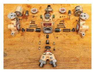
**Components of the Visor Selector Valve** The spare Visor Selector Valve, stripped down with refurbished components ready to be reassembled. *Photo: James Cullingham (concorde-photos.co.uk)*
