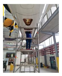
**Nose system** Peter Ugle fixing the connection on the nose jack to stop the leak. *Photo: Heritage Concorde*
