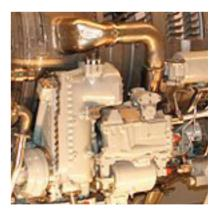
**Location of the SSP and FCU** Detail from a display specimen of the Olympus 593 engine. The large, lightcoloured component just below the right-angled pipe, just right of centre in this image, is the Flow Control Unit (FCU). The Second Stage Pump (SSP) is behind and attached to the FCU. *Photo: Nimbus227 / Wikimedia Commons (CC BY-SA 4.0)*
