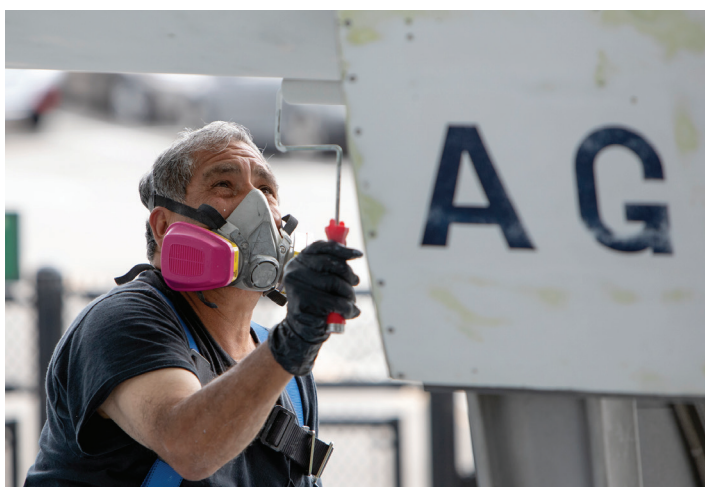
Painting in progress The aircraft had to remain in situ and could not be sprayed, so both large areas (top) and small corners (above) had to be painted by roller. Photos: Ted Huetter/The Museum of Flight
