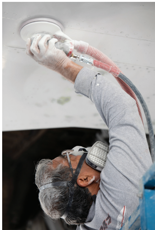
Minimising dust Right: A worker sands the underside of the aircraft. The vacuum tube for collecting the dust can be seen attached to the sanding pad. Photo: Ted Huetter/ The Museum of Flight
