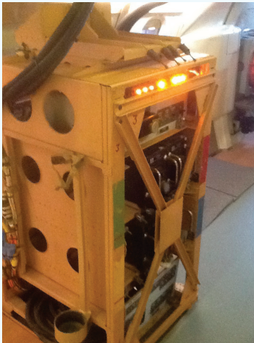
Test flight units The bulky cabinets holding the first digital Air Intake Control Units, installed in G-AXDN's cabin; these units are still in place today, and have been restored to show how they would have looked while in operation. Photo: John Dunlevy
