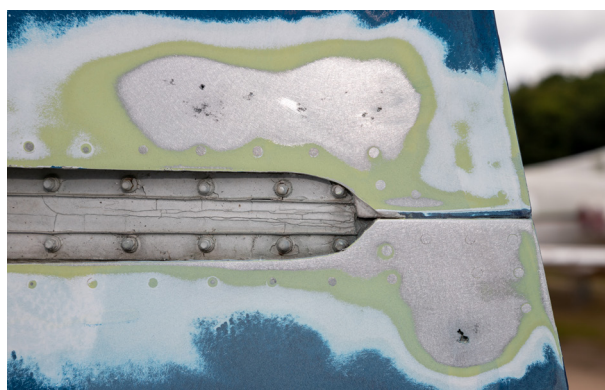
Right-hand mounting point with speed tape 'cover'. Photo: James Cullingham
