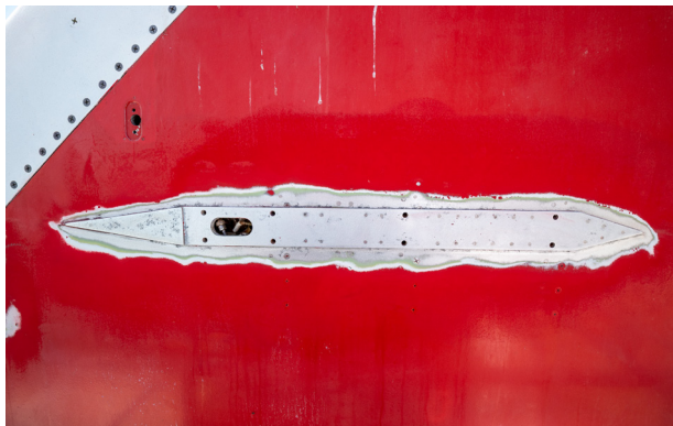
Left-hand antenna mounting point after initial clean-up. Photo: James Cullingham
