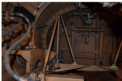
Inside the nose A view inside the nose (above). The curved runners for the visor mechanism (right); Heritage Concorde cleaned and greased the mechanism on the first day of work. Photos: Heritage Concorde
