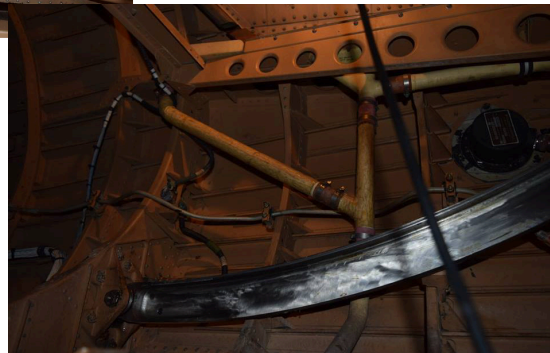
Inside the nose A view inside the nose (above). The curved runners for the visor mechanism (right); Heritage Concorde cleaned and greased the mechanism on the first day of work. Photos: Heritage Concorde
