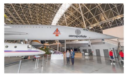
Aviation, who helped to develop Concorde's wing. He told us a little about the complex and subtle series of changes that had been made to the wing between the prototype and the production versions, in order for the wing shape to work at all speeds; apparently, just a slight re-shaping of the leading edge made the difference between the aircraft having a maximum safe speed of Mach 1.6 and Concorde flying effectively beyond Mach 2.
