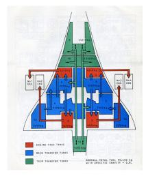
**Concorde fuel tank layout** Engine feed tanks are shown in red, main transfer tanks in blue, and trim transfer tanks in green. *Source: David Macdonald*
