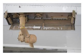
Ram Air Turbine (RAT) The RAT is seen in its "deployed" position under the starboard wing. Photo: David Macdonald establishes that engine response during a go-around is satisfactory.
