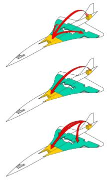
(shown in red on our diagram; see opposite page). Tanks 5, 6, 7, and 8, and tanks 5a and 7a, in turn supplied tanks 1 to 4. The fuel in the foremost and rearmost tanks – 9, 10, 11, and 12 – would be moved fore or aft to adjust the C of G.
